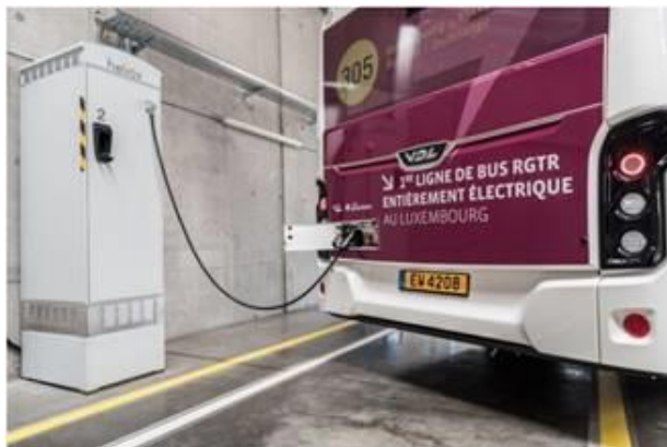
Figuur 20: Heliox 2x30 kW CCS charger in Luxemburg [16]
